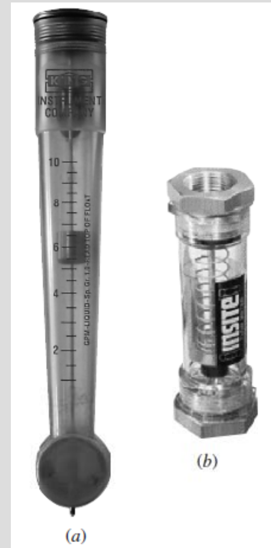
Two types of variable-area flowmeters: (a) an ordinary gravity-based meter and (b) a spring-opposed meter.
