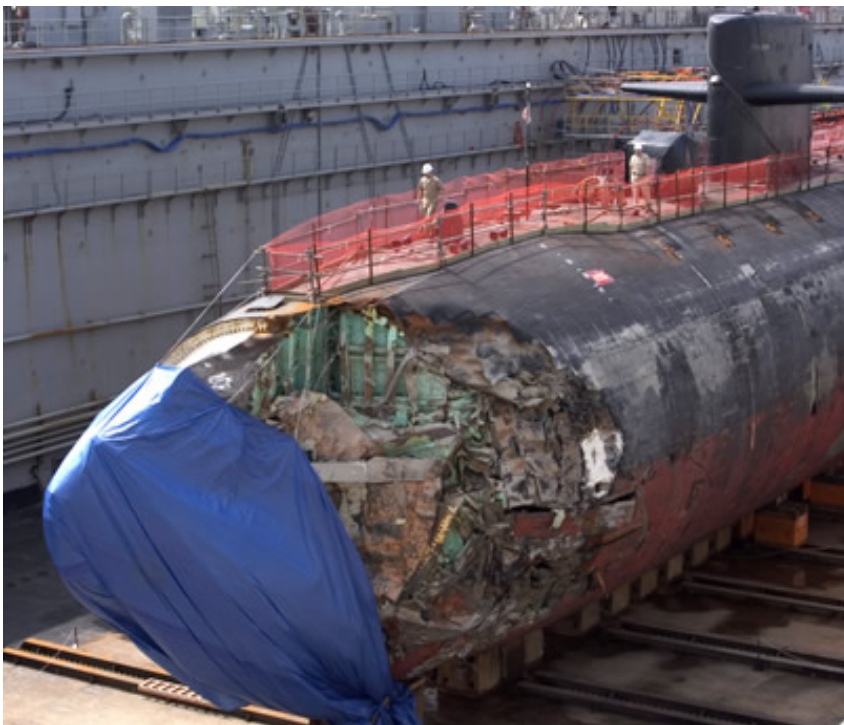
Damage to SSN 711 (USS San Francisco) after running aground on 8 January 2005.
